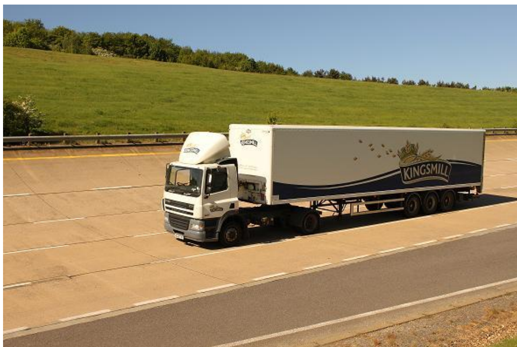
Figure C1. Test vehicle with cab deflector
