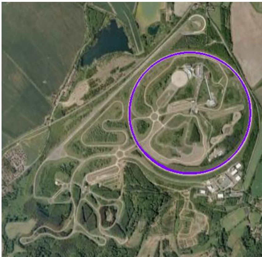
Figure 1. Millbrook high speed steady state route (circle diameter c. 1km)
