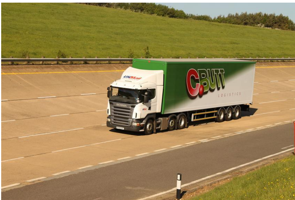
Figure C5. Test vehicle for low rolling resistance tyre tests
